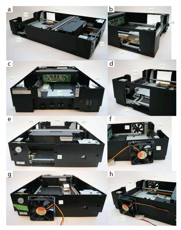
**Figure 3-2:** Photographs of chassis modifications. **(a):** The scanner chassis with its lid removed, and four cuts, H1–H4, made into its walls. **(b–e):** Close up views of each cut. **(f–h):** 8cm fans are glued into holes H1–H3.
