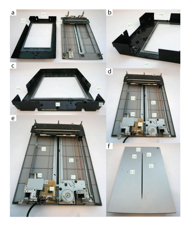
**Figure 3-3:** Photographs of mounted scanner fan. (a): The Transparency Unit (TPU) is shown with its top and bottom separated. (b-c): Three cuts, H<sub>5</sub>-H<sub>7</sub>, are made into the bottom of the TPU. (d): Four holes are drilled into the TPU lid, and (e) filled with machine screws. (f): The holes are shown from the top of the lid.
